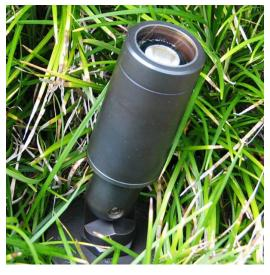
A separate, loose, cylinder with angled glare shield is also included for this fixture. When the fixture is shipped with the angled glare shield, it is in line with the axis of the knuckle. However the accompanying cylinder illustrates how the glare shield can be field-rotated by loosening the (2) side set screws.
